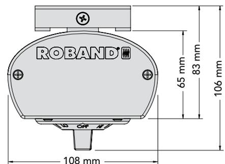
Dimensions for fabricator quartz lamps and infra-red heating assemblies (HUQ & HUE).
